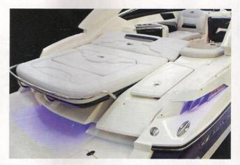
Note how the grab rail surrounding the aft lounge is below the level of the cushion. A detail other builders miss, this allows one to stretch out in comfort without skinning shins on the rail. The cabin's well-equipped.
