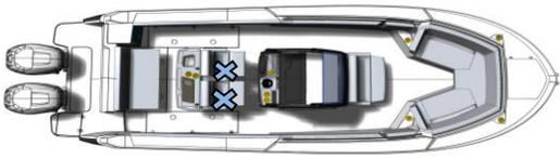
\* Ballast used to simulate weight of full fuel and water tanks and located on deck over fuel tanks
