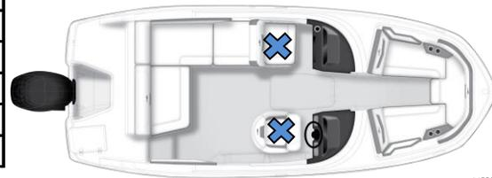
\* Ballast used to simulate weight of full fuel and water tanks and located on deck over fuel tanks
