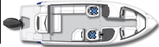
\* Ballast used to simulate weight of full fuel and water tanks and located on deck over fuel tanks
