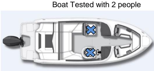
\* Ballast used to simulate weight of full fuel and water tanks and located on deck over fuel tanks
