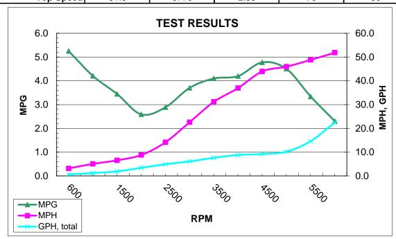
Notes: These test results are only valid for the boat listed by the hull ID#, at the time, date and place of the test. Testing variables include but are not limited to weather, prop, hull, and water condition, installation of various options, and captains. Speed was measured by GPS. Testing performed on fresh water near sealevel. Range is based on 90% of fuel tank capacity.
